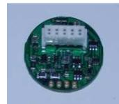
**OT-SC-IF** Sensor Connector Board – for use on Naked probe and in sensor cell testing
