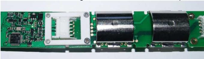
When all of the Sensor Cells and Connection Segments have been installed, connect the SDI-12 Concentrator board to the first sensor. Then fit two Connector Clips and secure with 4 screws.
