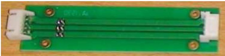
Working from left to right, push the plug on the bottom of the Sensor Cell into the Socket in the top of the next Sensor Cell or Connection Segment. Next place a Connector Clip on either side of the connector. Then fit two screws in from each side and tighten with a Number 1 Phillips Screwdriver.
