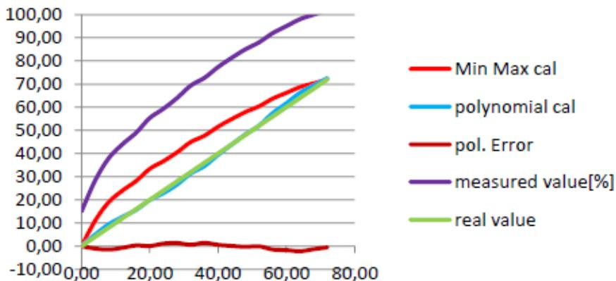
The graph above shows that the polynomial calibrated results show good matching with the real volumetric soil value. The maximum error is 2.2%. The graph also shows the error from the Min-Max calibration, which in this case is less accurate due to the non linear behaviour of potting soil.
