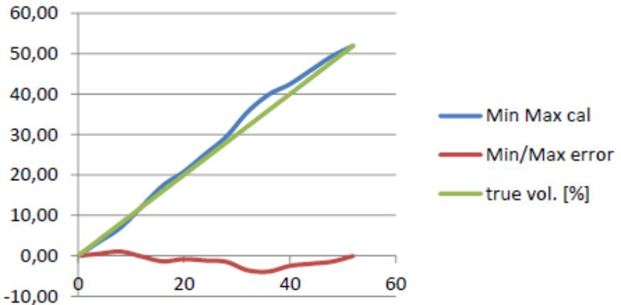
The maximum error magnitude depends on the soil type. In soil types with mainly mineral content such as sand, the measurement response of the probe is close to linear and a Min/Max calibration results in a good approximation to the real volumetric soil moisture value which is accurate enough for most applications.
