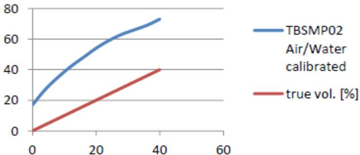
An Air-Water – calibrated Otto SMP will respond with 26% in dry sand and with 86% in fully saturated sand. The corresponding, true volumetric values would be 0% and 40% however.
