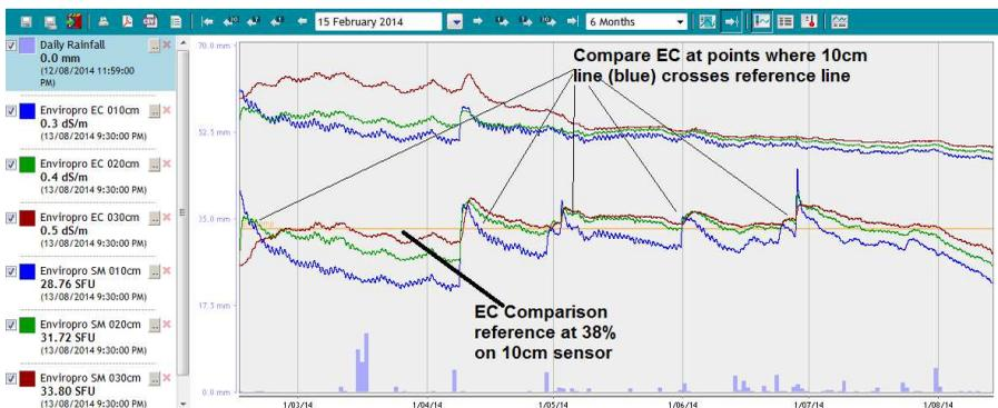
The above picture shows data from the 10, 20 and 30cm soil moisture and EC sensors for a 6 month period with the EC sensors at the top and soil
