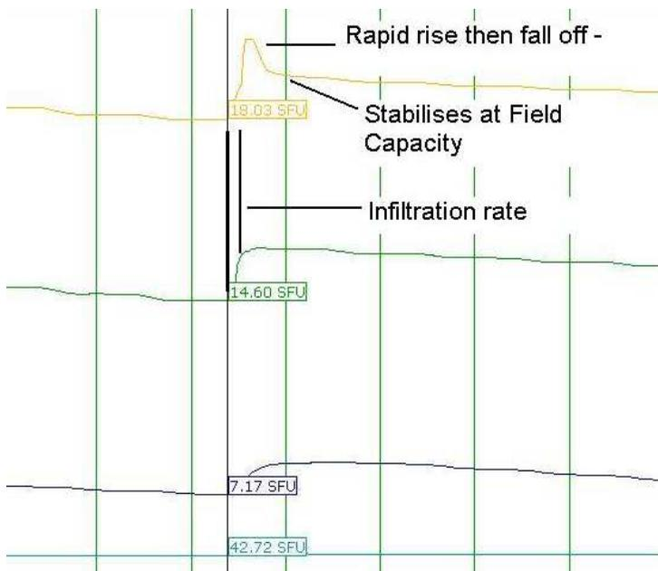
In the above graph, the water reached the third sensor but not the 4<sup>th</sup>. The top sensor rises quickly at the start of irrigation and then, at the end, falls off quickly with drainage. The water level then stabilises at field
