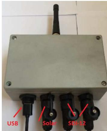
The TBSL1 connects to a PC using a USB connection, You can connect to the Type A connector on the case or, with the case open, to the Type B (printer style) connector on the PCB.
